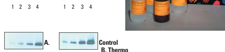
Figure 4. Immunoblot analysis of GST by chemiluminescent detection after Thermo Scientific Pierce Reversible Staining, destaining and stain reversal. Different amounts of purified GST protein were applied to two 10% Tris-glycine SDS-polyacrylamide gels and electroblotted to nitrocellulose membranes. The control membrane ( Panel A ) was not treated. Panel B was subjected to the staining, destaining and stain-erasing protocol of the Pierce Kit. Both membranes were probed with anti-GST incubated with goat anti-rabbit IgG-HRP conjugate and detected using SuperSignal West Dura Substrate (Product # 34075). Lane 1. 125 pg, Lane 2. 250 pg, Lane 3. 500 pg and Lane 4. 1 ng.
