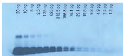
Figure 9. Lumi-Phos Substrate provides high sensitivity and low background. Serial dilutions of recombinant mouse IL-2 were separated electrophoretically on a 4-20% SDS-polyacrylamide gel. The separated protein
