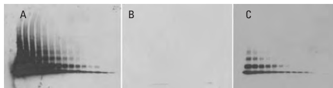
Figure 2. Antibody optimization study. Western blots of Interleukin-2 (diluted 20-0.156 ng) were detected using SuperSignal West Pico Chemiluminescent Substrate. The first blot (A) used the primary antibody diluted to 1:1,000 (0.5 µg/ml) of Rat Anti-Mouse IL-2 (BD PharMingen; San Jose, CA) and the horseradish peroxidase (HRP)-labeled Goat Anti-Rat secondary antibody (Product # 31470) diluted 1:5,000. The same blot was stripped with Restore Western Blot Stripping Buffer (B) for 5 minutes at room temperature and re-probed (C) with the primary antibody at 1:5,000 and the HRP-secondary conjugate at 1:20,000. SuperBlock Blocking Buffer was used for blocking.
