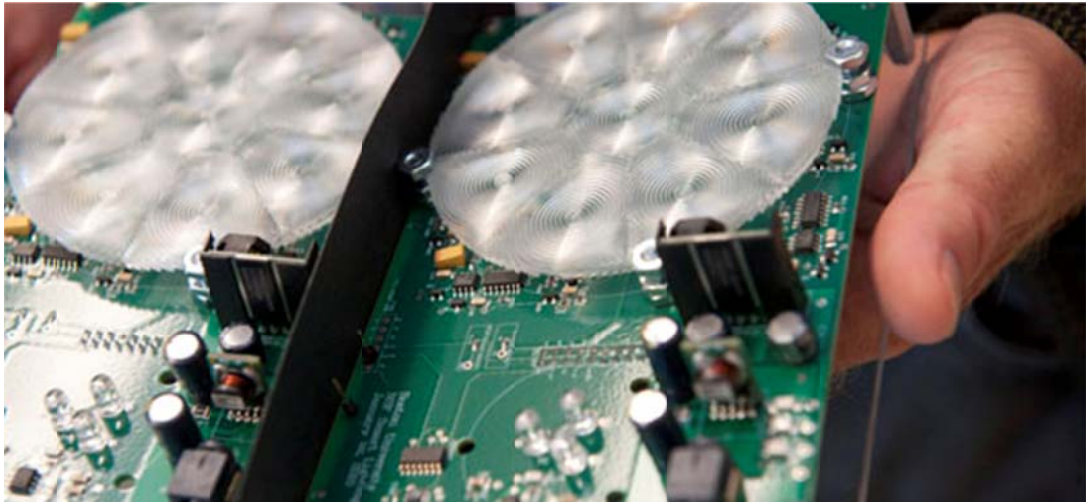
Fig 2: Web-Enabled LED lighting Prototype
