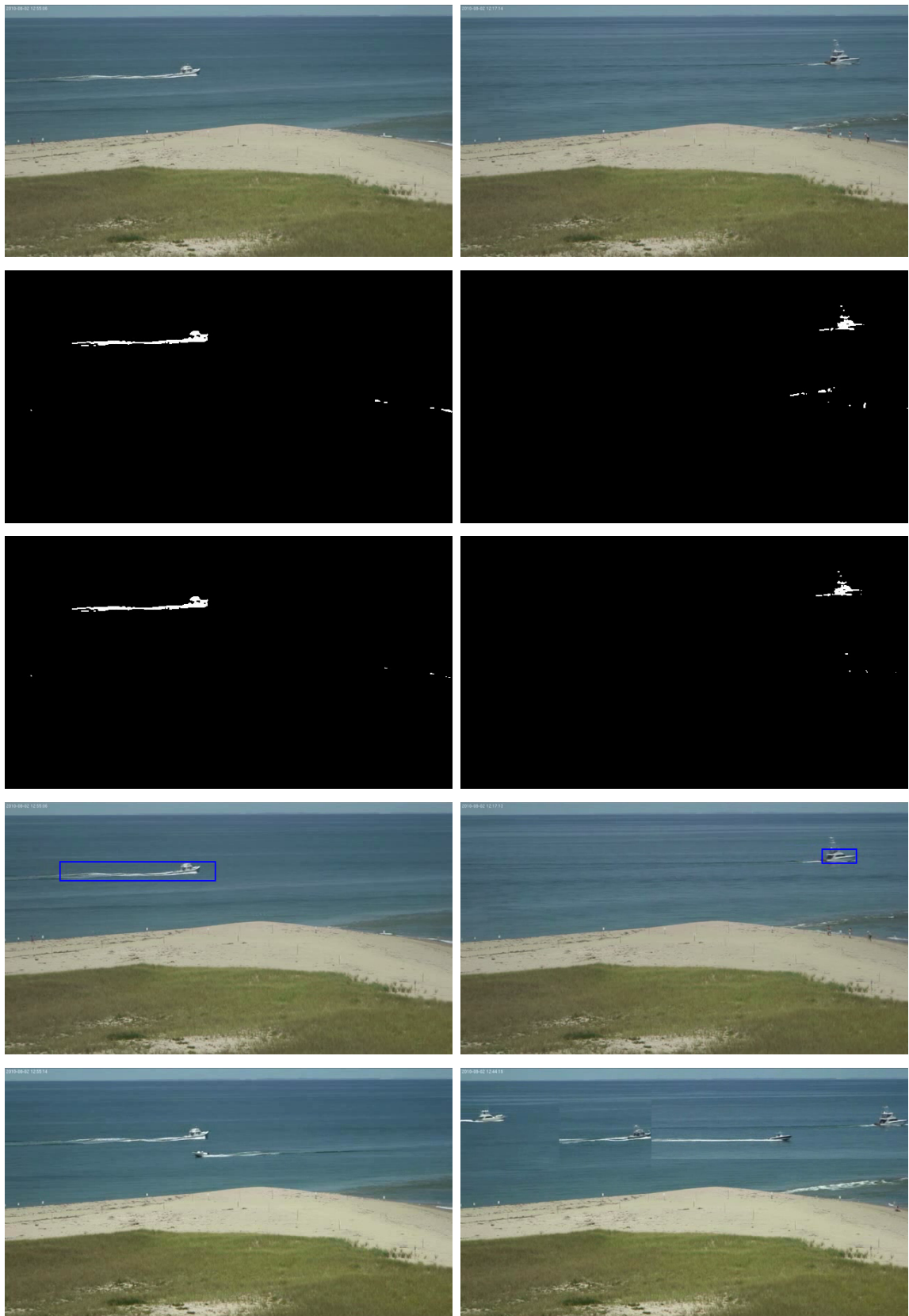
Figure 18: Samples of typical input video frames (top row) and outputs from the processing blocks in Figure 11: (row 2) background subtraction, (row 3) behavior subtraction, (row 4) object detection, (row 5) video condensation.
