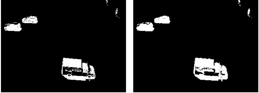
Figure 12: Background-subtracted frame before (left) and after (right) enabling the Markov random field (MRF) model. Notice that the MRF model helps to “fill in” the interiors of the silhouettes of the cars, the truck, and the pedestrians.
