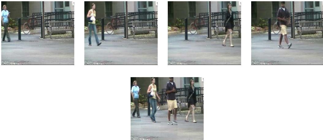
Fig. 13 Condensed Outdoor traffic video: four original frames (top) and one condensed frame (bottom)
