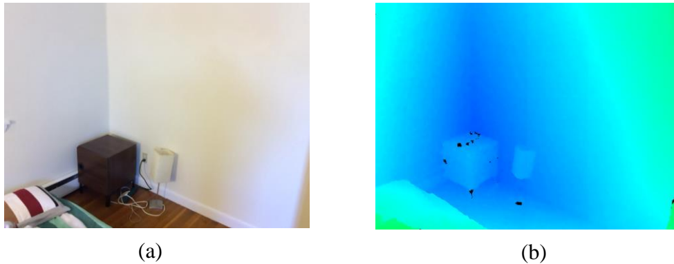
Figure 4 (a) Image of a room with a corner between two walls being the furthest points of the scene from the camera, and (b) the corresponding depth map (dark blue indicates large depth).
