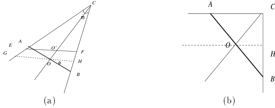
Figure 9: (a): Determining the position of the plane of rectification OG = \frac{w \cos \varpi}{2 \cos(\phi + \varpi)} , OH = \frac{w \cos \varpi}{2 \cos(\phi - \varpi)} (b): Situation when a projection of an image onto a finite plane is impossible
