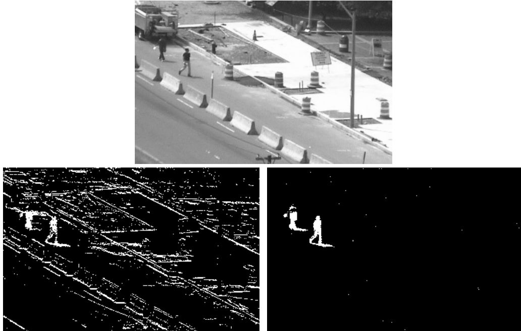
Figure 4.7: When camera shake is present, the background subtraction result can have a high number of false detections when using \mathcal{M}_1 (left). Performing realignment on the frames before modeling takes place mitigates most of these errors (right). Details of the realignment technique used can be found in Appendix A.
