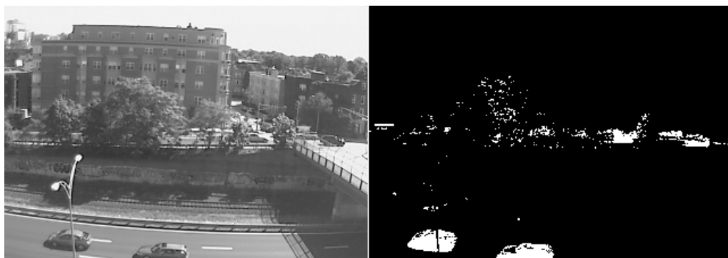
Figure 4.4: Although the cars on the highway below are well detected, the trees in this frame, whose leaves and shadows thereof displace slightly, are incorrectly detected as moving objects using model \mathcal{M}_0 .
