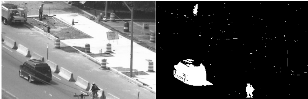
Figure 4.11: Describing a pixel by the content of a region can ‘over-model’ the background in some cases, resulting in large missed foreground regions. A portion of the roof of the van is incorrectly labeled as background with \mathcal{M}_2 because it resembles a nearby region of the scene.
