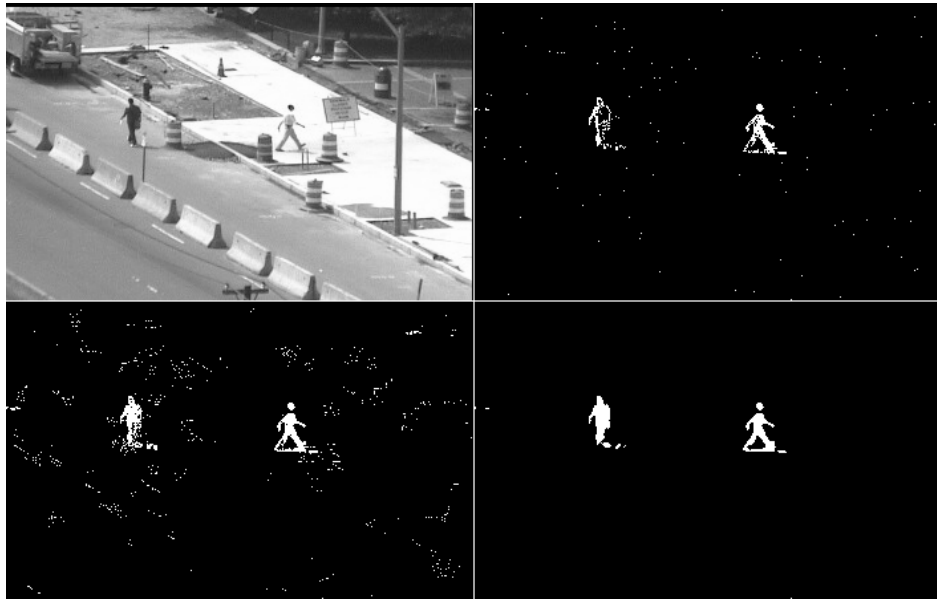
Figure 5.9: Background detection result on sidewalk sequence. Thresholding of P_{\mathcal{B}} (LIT model) alone (top right), inclusion of P_{\mathcal{F}} (bottom left), and final MRF step (bottom right).
