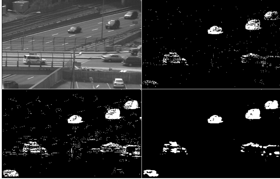
Figure 5.8: Background detection result on highway sequence. Thresholding of P_{\mathcal{B}} (LIT model) alone (top right), inclusion of P_{\mathcal{F}} (bottom left), and final MRF step (bottom right).
