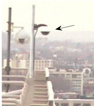
Figure A.1: Roof-mounted PTZ camera used to capture image sequences.
