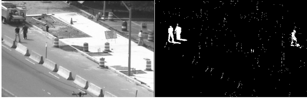
Figure 4.8: Although image preregistration will greatly improve the detection performance using \mathcal{M}_1 , occasional misregistration may still result in detection errors along edges.
