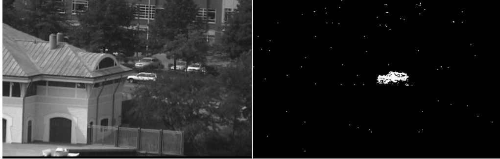
Figure 4.6: The trees in this sequence move slightly with the wind, however \mathcal{M}_1 is able to sufficiently model the dynamic background. The resulting detection mask highlights the moving object of interest, the car, and not the unimportant motion of the trees.
