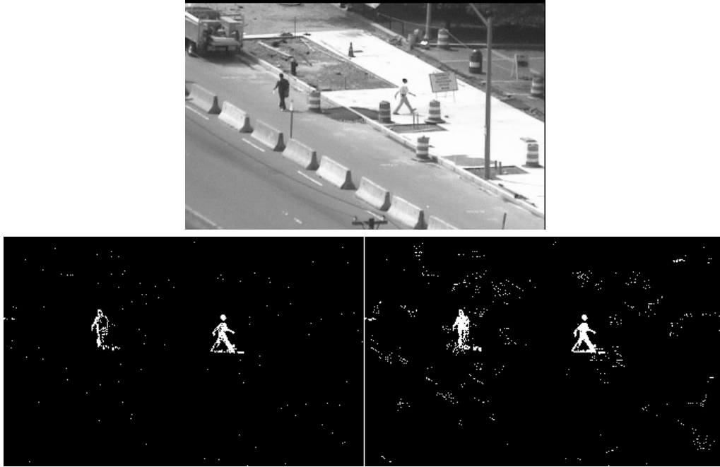
Figure 5.3: A single frame from the testing sequence sidewalk (realigned from a shaky camera) and detection results below. The initial detection result after thresholding P_{\mathcal{B}} (LIT model) on the left and the effect of utilizing foreground modeling in the detection process to the right.
