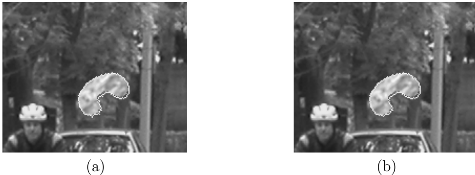
Figure 8.1: Results for the M-frame MD algorithm, applied to the synthetic image sequence Bean : frame #15 from the sequence overlaid with final boundary calculated using the (a) standard level-set implementation and (b) fast level-set implementation.
