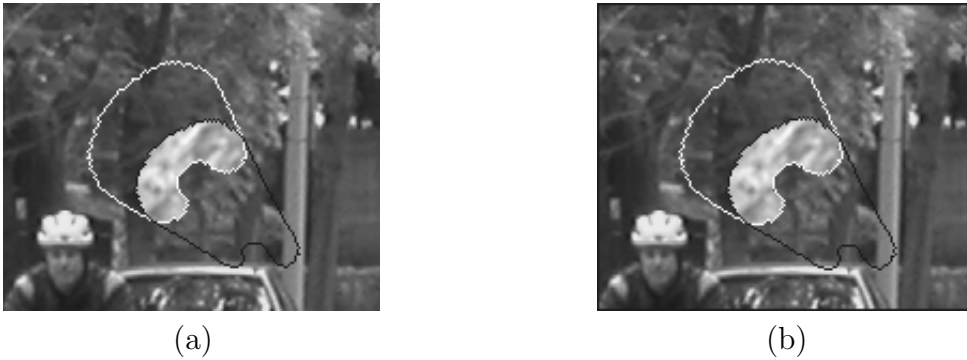
Figure 8-4: Results for the M-frame MCS-B algorithm, applied to the synthetic image sequence Bean : frame #20 from the sequence overlaid with final boundaries calculated using the (a) standard level-set implementation and (b) fast level-set implementation.
