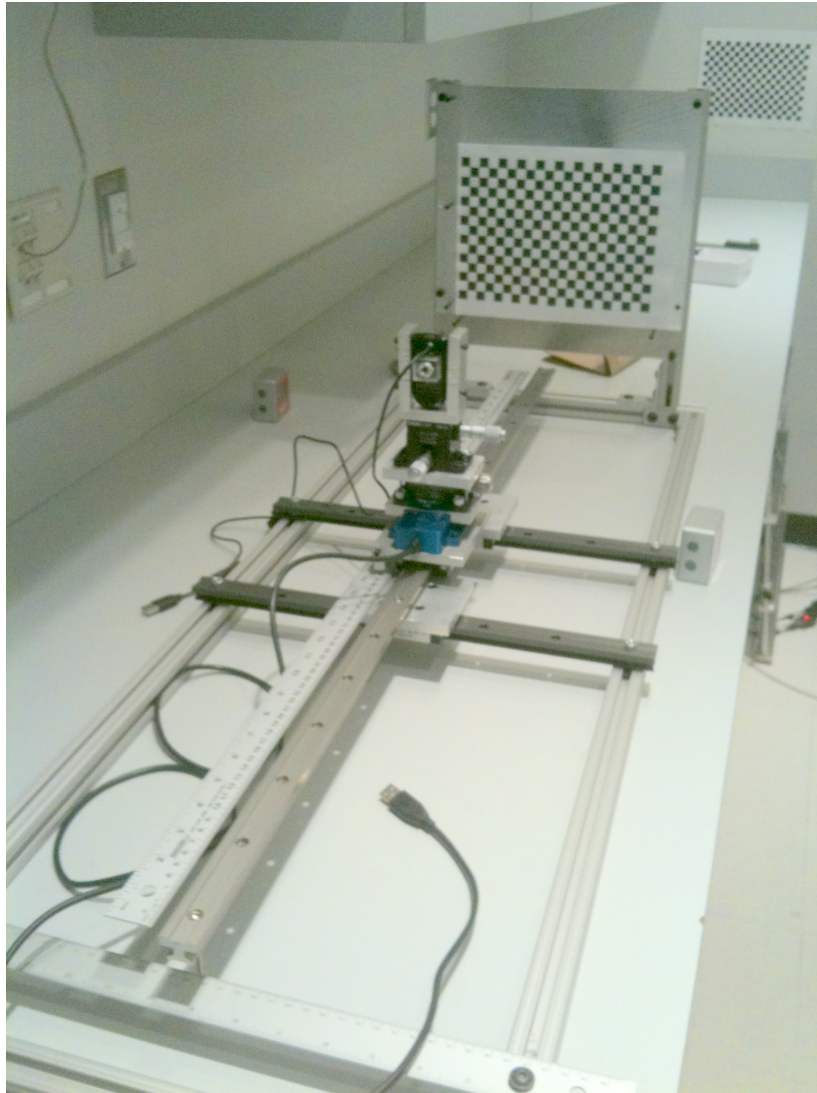
Figure 6-46: Mechanical platform developed to allow precise camera translations and rotations.
