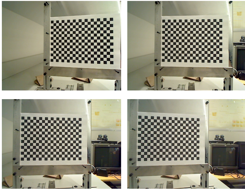
Figure 6-50: Sample frames from a video captured while rotating the camera around y -axis.
