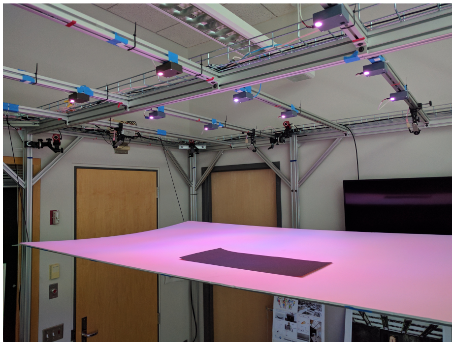
Figure 2-9: Photo of our testbed with the 64x flat object. Due to the limited intensity of light sources, we hang a board in mid-air as a proxy for the floor and thus to increase the reflected light intensity.
