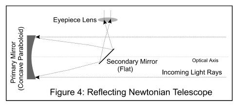
The first telescope design that used mirrors instead of lenses was invented by Isaac Newton in 1680. The objective in this design (see Figure 4) is a concave parabolic mirror. which reflects light onto a flat secondary mirror, moving the focus of the primary outside of the path of the light entering rays the
