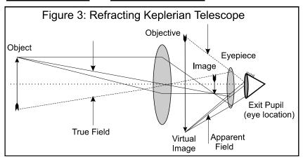
Telescopes Types - A refracting telescope is shown schematically in Figure 3. In 1609, Galileo Galilei
