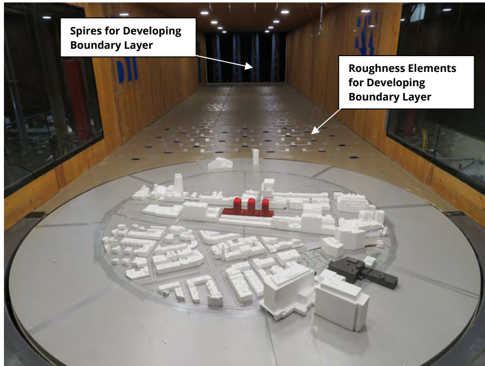
Image 1: Photograph of Scale Model in RWDI Boundary Layer Wind Tunnel
