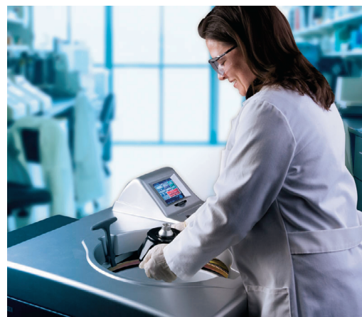
Figure 1 Some rotors can be removed without being opened, meaning they can be moved to a safety cabinet and opened under safe conditions.
