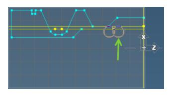
The circle selected will be drawn and a connector point will be created between the circle and the line. When tangent features are created they will create connector points when possible.
