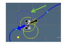
11. Click the arrow pointing right to create the toolpath for a clockwise contour.
