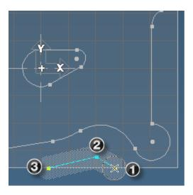
Points are created wherever you click the mouse, and a line will be drawn between the points created. All geometry created using this method is fully connected; the endpoints of the contour are terminators and the points between lines are connectors. You want to make sure the path of the tool covers the area of stock we need to rough.
