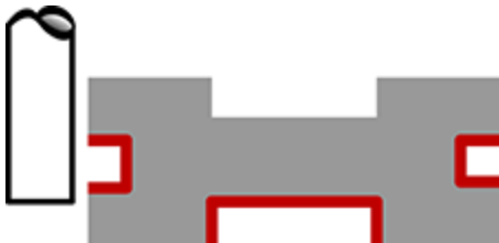
Areas of a part that may cause undercut problems
