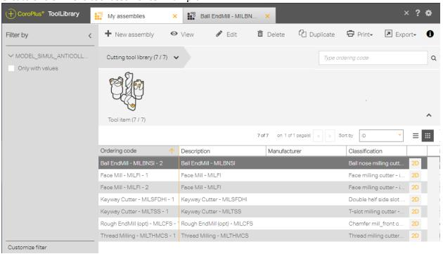
*Note:* You can create individual tool assemblies manually using New assembly, or you can subscribe to one or more assortments in a CoroPlus Catalog.
