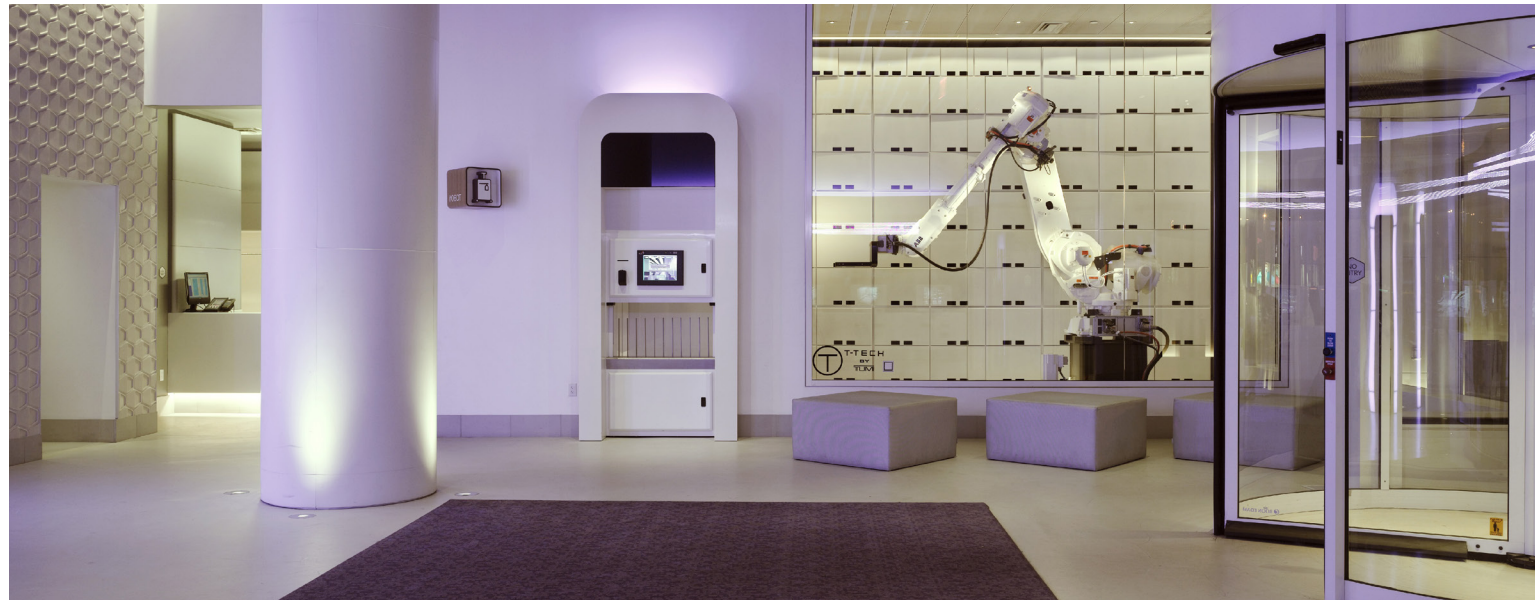
Among other futuristic features, the Yotel New York has an automated check-in service complete with a robotic arm that lifts customers' luggage into storage bins.
