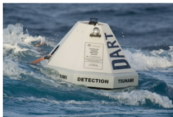
DART® - ETD buoy system Deep Ocean Assessment of Tsunami (DART) Easy to Deploy (ETD)
