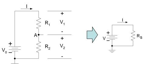
$$V_0 = V_1 + V_2 = IR_1 + IR_2$$
