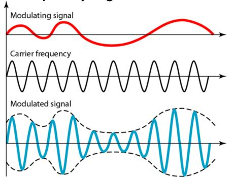
In VLC Signals, optical intensity is modulated.
