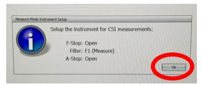
After the application is loaded there will be a pop up for F-stop and A-stop). Make sure the F-Stop and A-Stop is
