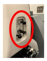
open (push knobs in) and the filter is set to F1 (measure) as shown on above. Select ok.
