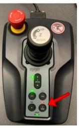
3) Set Z-stop (button on Motion Controller from blinking red to red)
