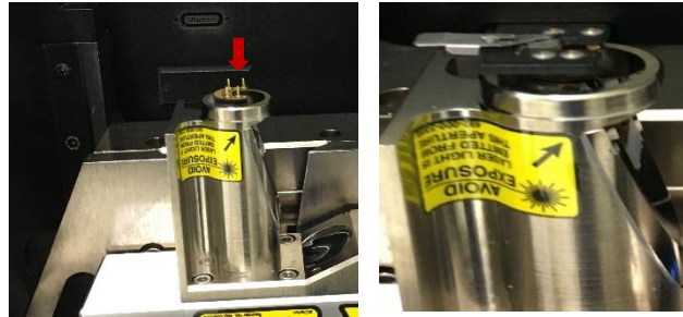
Figure 3: AFM head pin to insert cantilever holder, right panel: head after holder inserted
