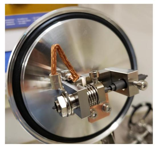
Press **Power** button on the front panel. Pumping starts automatically. There should be no hissing or gargling sound from the system, which indicate a leak. In case of the hissing/gargling noise from the pump, turn the power off and recheck the O-ring seal. Close the top cover plate gently ensuring a tight seal and begin pumping. Press power off after 15-30 sec of pumping and restart pumping. Repeat this step 3-4 times to purge the lines and to achieve a better vacuum level.
