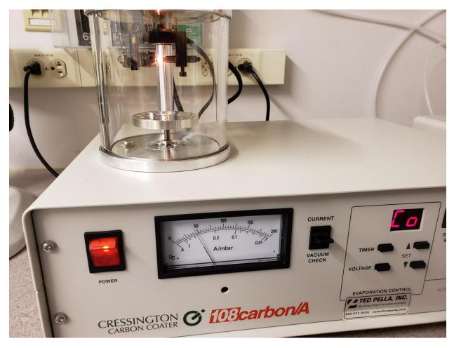
Observe current values during deposition. Typical currents close to 50 A are suggested for high quality coatings. Higher currents will result in heating but no carbon evaporation as well as carbon rod and assembly failure.
