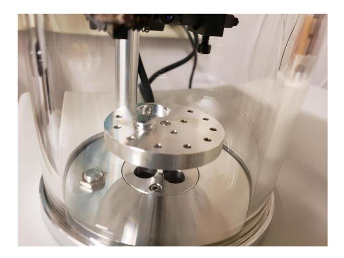
Lower the top plate **slowly** onto the glass jar to ensure a vacuum seal:
