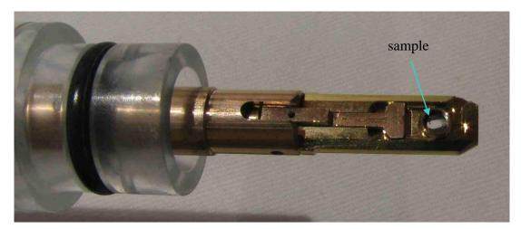
If either of these items appears to be loose, stop, it is not safe to put the holder into **TEM.** Try repeating the specimen loading procedure.
