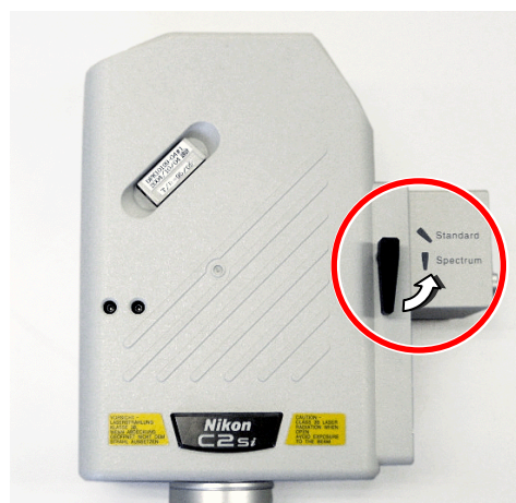
Figure 5.3-22 Switching the optical path of the C2 scan head
