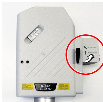
Figure 5.3-1 Switching the optical path of the C2 scan head
