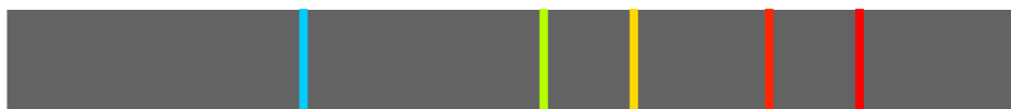
Colors of five different light emitting diodes (LED's). The horizontal axis is wavelength, increasing to the right.
