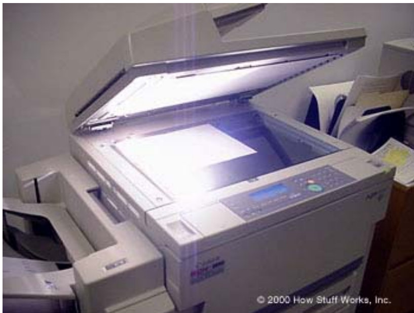
A strong lamp illuminates the sheet of paper to be copied.
